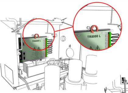
Single screw removal of trigger module
